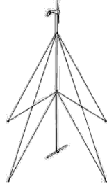
Figure 40: Tower with guy wires
