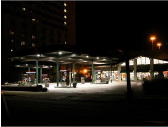
Figure 35: Recessed (full cutoff) service station lighting on the left; surface mounted (non-cutoff) on the right.
