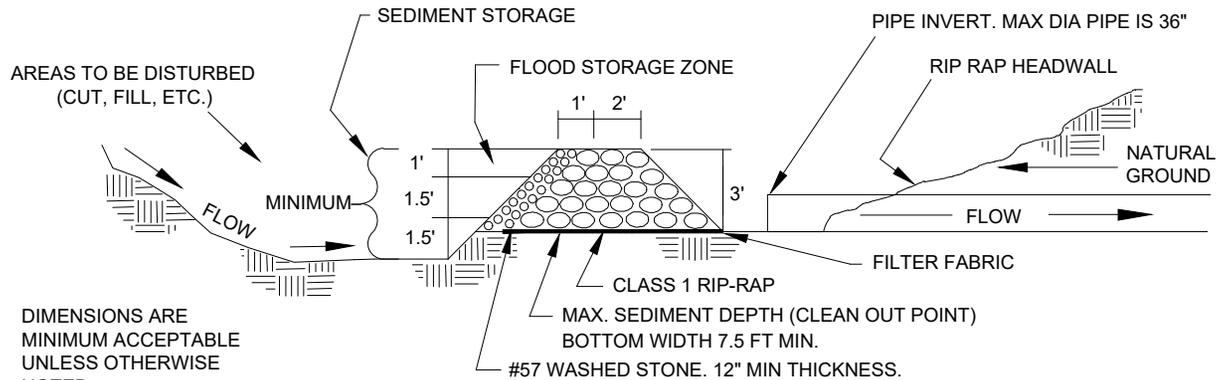
**SECTION THRU BASIN, FILTER AND CULVERT PIPE**
