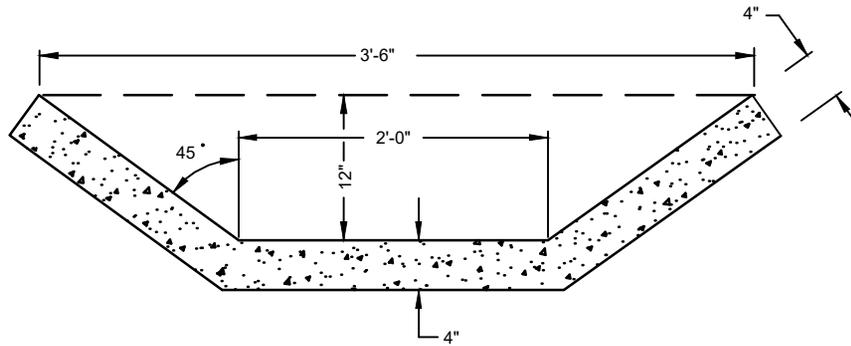
SLOPE DRAIN, BASE DITCH OR BERM DRAINAGE
