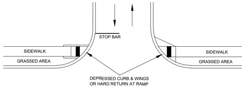
FOR RAMPS AT ASPHALT TO ASPHALT STREET TYPE DRIVEWAYS OR PRIVATE STREET TIE IN.
