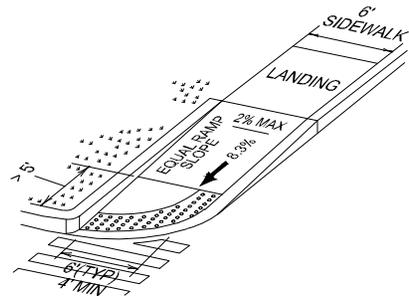
CROSS SLOPE NOT TO EXCEED 2% ON ANY PORTION OF RAMP OR TRANSITION TO STREET.
